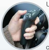
Unlike a conventional steering ball there is no separate fixed position keypad. The smartSTEER integrates control of the steering and operation of secondary
