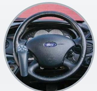
The design of the **smartSTEER** is ergonomic and robust to provide assured and safe control whilst also offering variable positioning on the steering wheel for maximum comfort. The **smartSTEER** has an automatic dimming handset and can be quickly released from the steering wheel when not in use, or when the vehicle is left unattended.
